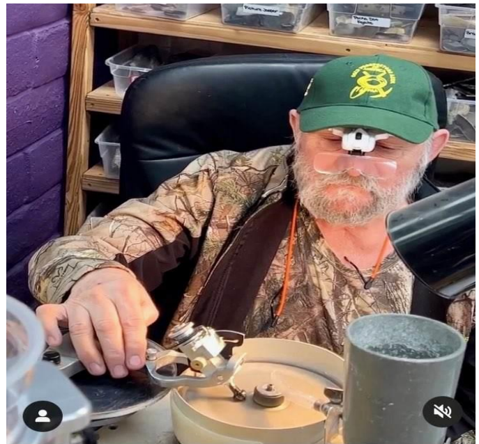
Here, I am using an old Raytech-Shaw faceter. I had contacted the manufacturer last week in the need of new Dop sticks and they were able to get me a new set in just a few days. It was quite an education for the first time setting up and using my old machine.
